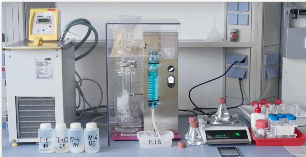
FIGURE 3. The semi-miniaturized Polydest steam still (with protective shield) is shown in the laboratory setting.
